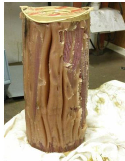
Filter blockage due to high Cloud Point
