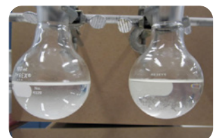
Figure 10: Test start: T= 48H Left flask: fuel + cat fines Right flask: fuel + cat fines + Aderco 2055G*
