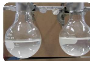
Figure 9: Test start: T= 24H Left flask: fuel + cat fines Right flask: fuel + cat fines + Aderco 2055G*
