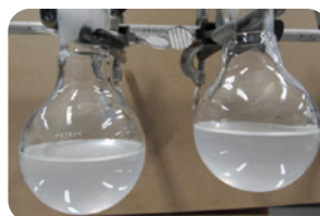
Figure 8: Test start: T= 0 Left flask: fuel + cat fines Right flask: fuel + cat fines + Aderco 2055G*
